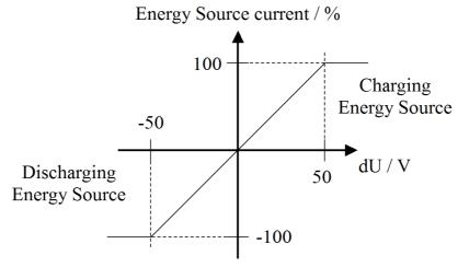
DC-Link voltage reference model: dU = measured voltage - voltage reference) Energy Source voltage reference model: dU = voltage reference - measured voltage
